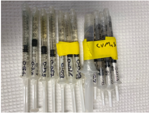
Figure 15: Phantom samples of MnCl 2 and CuS-Mn NP. Mn concentration was in the range from 0.0mM-0.54mM.
